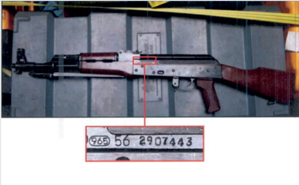
Figure 2 Chinese-manufactured Factory 965 Type 56 assault rifle
